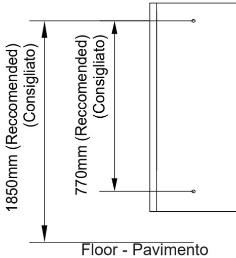
Drill 2 holes (Distance is 770mm) in desired position.
